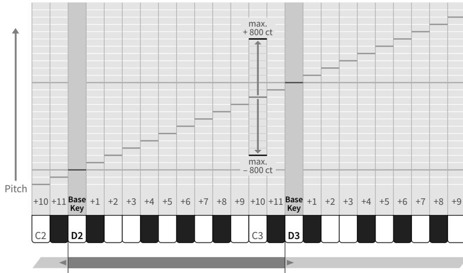
A scale where four keys have been micro-tuned:
