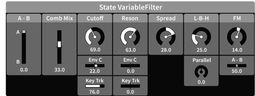
The State Variable Filter has a variable 4-pole structure with:
