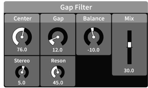
A 4-pole lowpass and a 4-pole highpass in a parallel or serial structure, creating a flexible band-rejection or band-pass filter. The offset between the center frequencies of the left and the right channel can be controlled.
