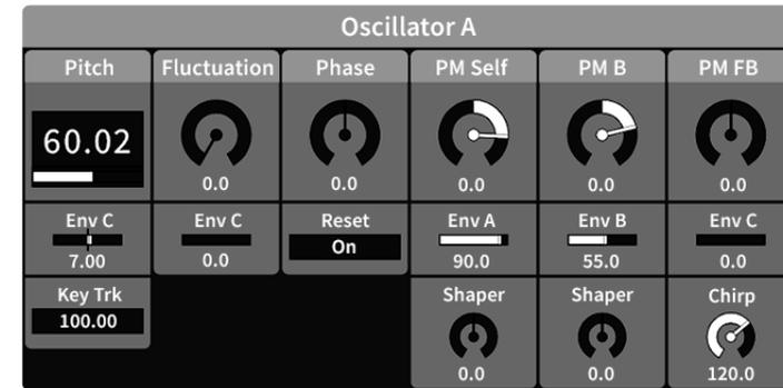
The two sine wave oscillators are the only signal sources. With a random frequency fluctuation they can also produce tunable noise. They are equipped with three phase modulation inputs for:
