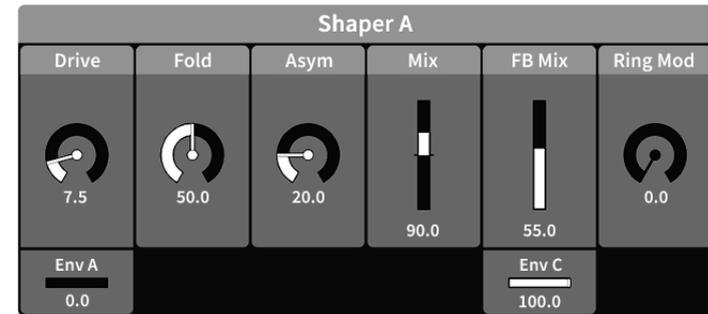
The signal of each oscillator is processed by a wave shaper. The shaping curve is a sine function with adjustable foldback and asymmetry. The mix amounts of the shaper signal can be adjusted individually for each phase modulation branch and for the output.
