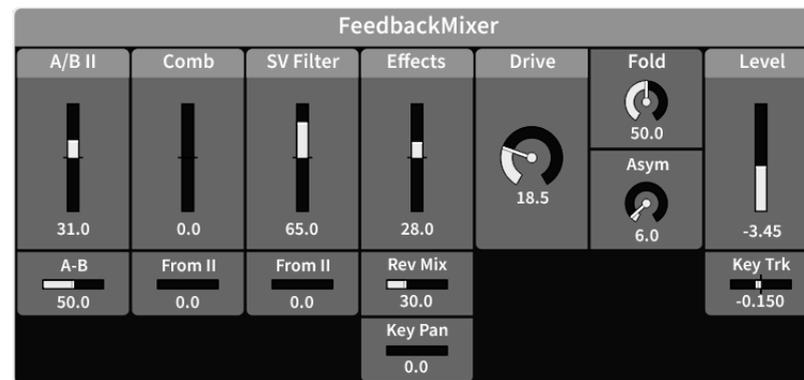
This mixer combines the following signals for the feedback bus: the outputs of the Comb Filter and the State Variable Filter and the output of the Effects chain, with a separately adjustable amount of Reverb. It includes a sine shaper for the sum signal.
