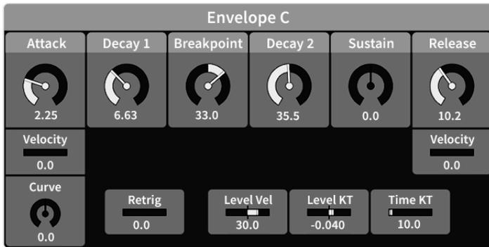
The third ADBDSR envelope has bipolar Breakpoint and Sustain levels. It can modulate:
