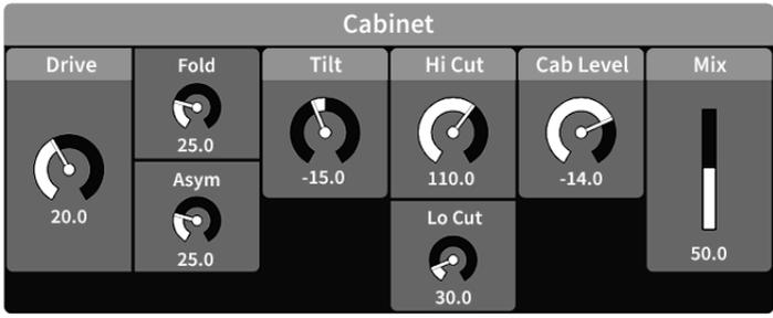
A stereo distortion unit (sine shaper) with pre and post filtering that can sound similar to a guitar amp driving a speaker.
