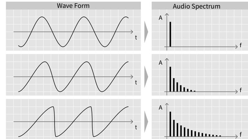
Oscillator signal without self modulation and different amounts of fluctuation:
