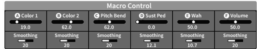
Six Macro Controls (A, B, C, D, E, F) are available as modulation sources. 106 parameters can be assigned as modulation targets with individual amounts. For each Macro Control a Smoothing time can be set.
