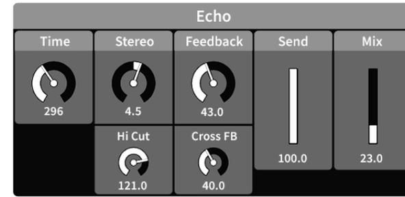
A stereo delay effect with adjustable cross-feedback.
