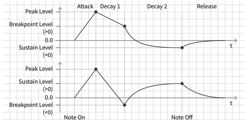
Envelope C - "Retrigger Hardness" Parameter (in monophonic mode):
