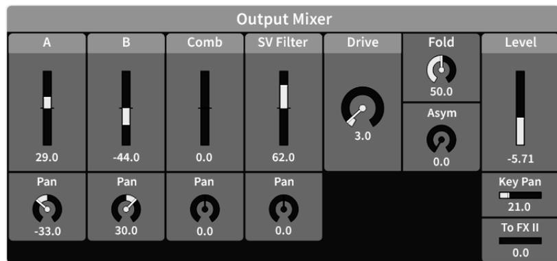
The Output Mixer creates a stereo sum of the signals from Oscillator/Shaper A and B, the Comb Filter and the State Variable Filter. It includes a sine shaper for the sum signal of each voice.
