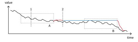
Normally, for fast and wide enough value changes, the track-and-hold mechanism is in "track" mode and the output strictly follows the momentary input (black).
