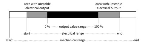
The measured electrical range can only increase over time of usage and once it is large enough for a successful scaling -- larger than about 1/4th of maximum range -- the pedal actually starts to produce output values. The only way to make the used electrical range smaller again is to reset the pedal.
